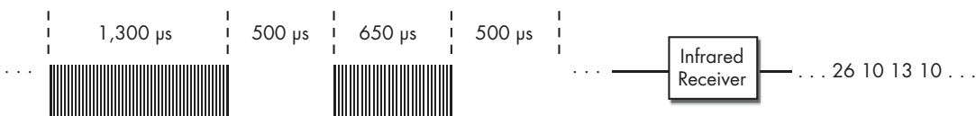
Figure 12-8: Measuring waveform timing in external hardware
