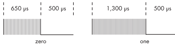
Figure 12-3: Modulated pulses in the Sony TV protocol
